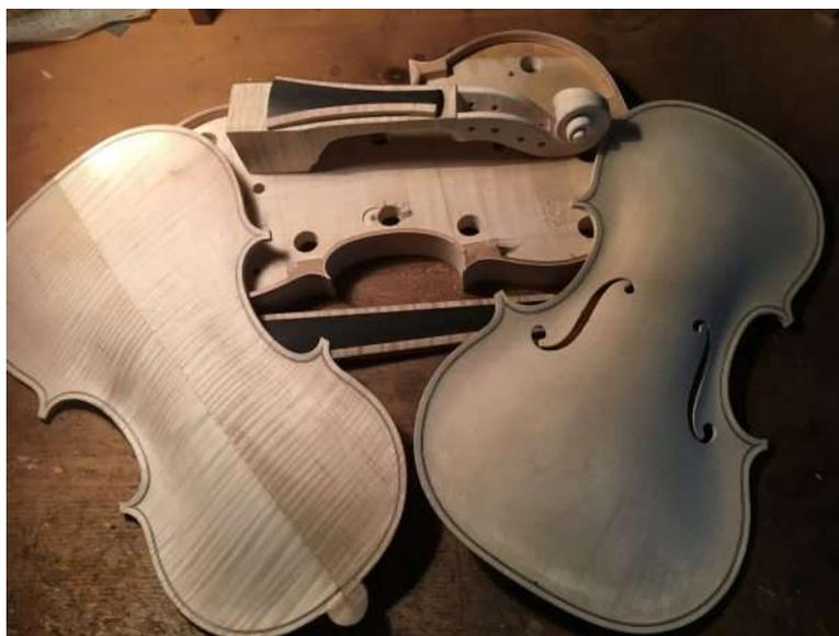
*Figure 3 Parts are ready for final assembly. Fluting is just visible in the shadows of the belly or top plate (right).*
