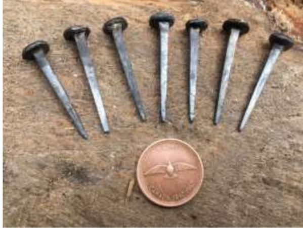
*Figure 1 Custom-made nails by Graeme Sheffield. Only three nails are needed to attach the neck to the violin body*
