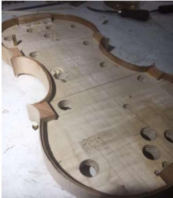
*Figure 2 Rib structure on a mould. At the very top, a through rib strengthens the neck-to-block attachment.*
